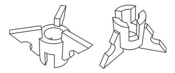
A UNION of three solids (a cylinder of diameter 20 units, a cuboid of side 20 units, and a Q.09 triangular prism with base of the triangle 20 units and height 20 units) is shown below. Visualise the new solid formed by the INTERSECTION of these three solids in this arrangement. How many surfaces will the resultant solid have?
